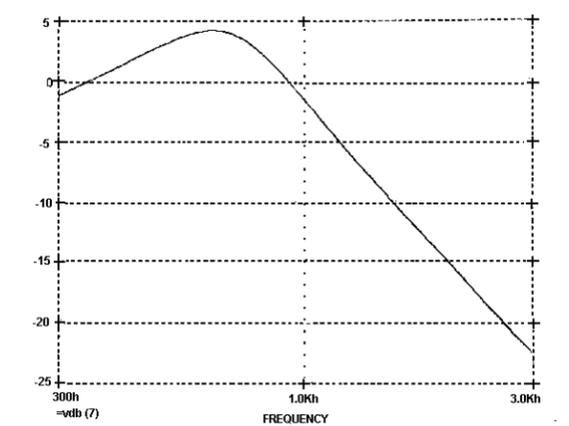
Figure 4 - Battery Alarm/Morse Code Band-Pass Filter
