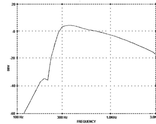
Figure 1 - Channel Guard Tone Reject (+1, -3 dBV)
