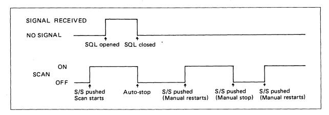
4. By setting the SCAN-STOP FUNCTION SWITCH in EMPTY position and the SCAN-STOP TIMER Switch in ON position, the scan will stop on an empty channel, then will restart after specified time is passed, whether a signal has been received or not.
