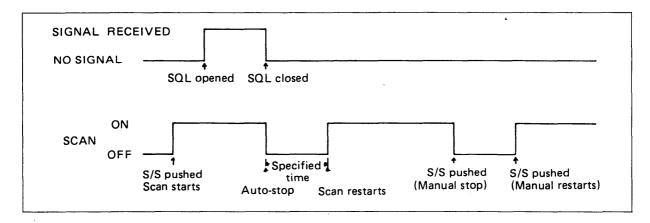
Set the SCAN-STOP TIMER Switch, SCAN-STOP INTERVAL Switch, and SCAN-STOP FUNC-TION SWITCH as to your own choice.
