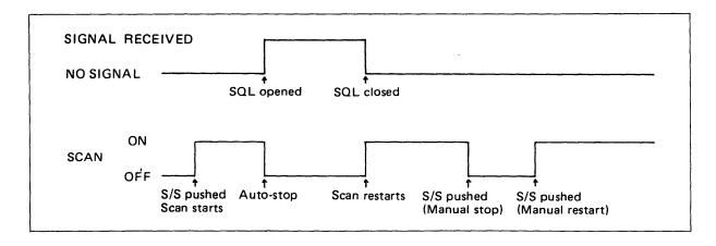
2. By setting the SCAN-STOP TIMER Switch in ON position and the SCAN-STOP FUNCTION SWITCH in BUSY position, the scan will stop on a signal, and will restart after specified time is passed, whether a signal has been received or not. The scan stop time is selectable 3 seconds (SHORT) and 9 seconds (LONG) with the SCAN-STOP INTERVAL Switch located under the access cover.
