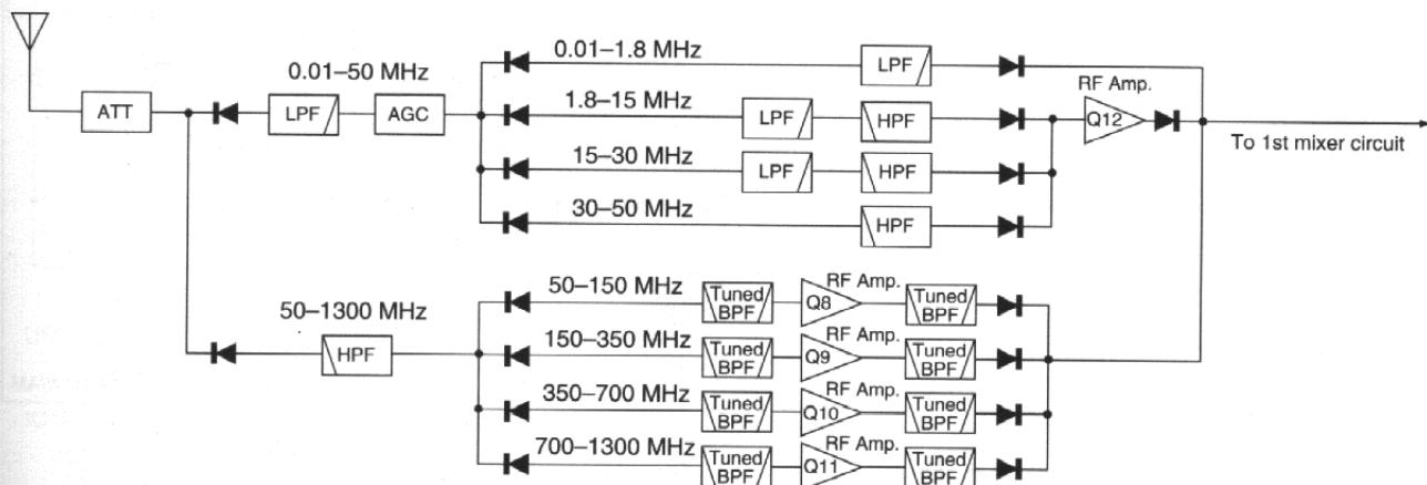
The 15–29.999999 MHz signals pass through the low-pass filter (L10, L11, C33–C37) and high-pass filter (L11, L12, C38–C42) between the band switching diodes (D3, D7), and are then applied to the 1st mixer circuit via the RF amplifier circuit (Q12).
