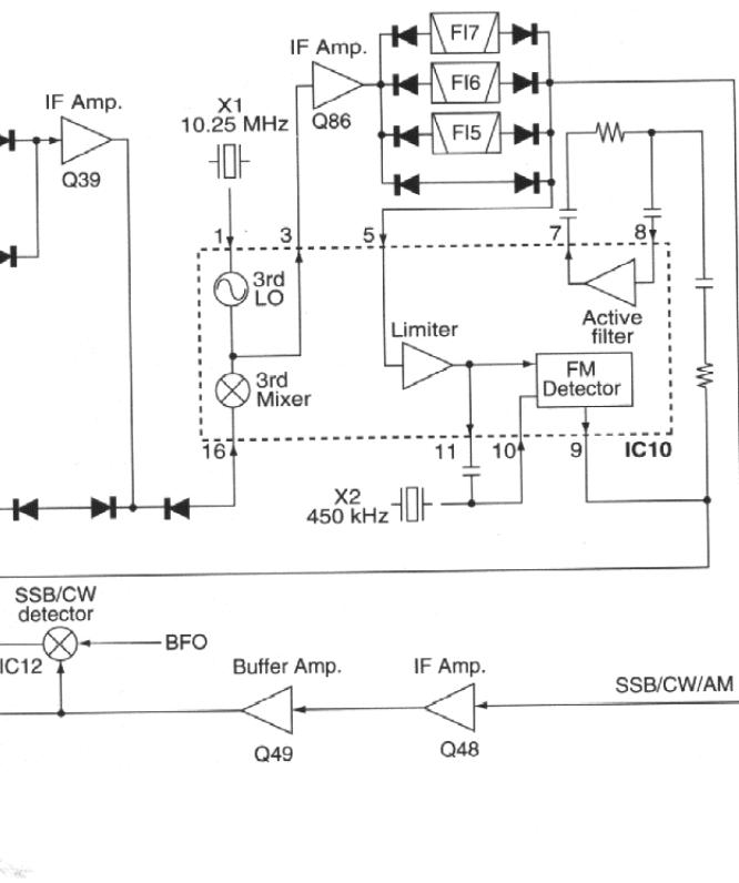
The 10.7 MHz 2nd IF signal from the buffer amplifier (Q39) is applied to the 3rd mixer section in the FM IF IC (IC10, pin 16). The applied signal is mixed with a 3rd LO signal generated by X1 (10.25 MHz) to produce a 450 kHz 3rd IF signal.
