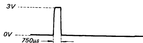
(BE) 0V DC WHEN AM SWITCH IS PRESSED TWICE OR a1 THROUGH d8 SWITCH IS PRESSED ONCE, MOMENTARILY ONE PULSE.
