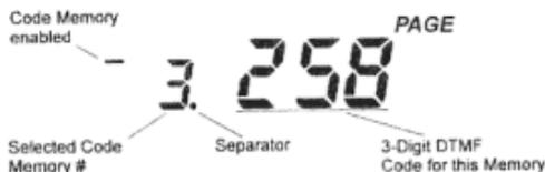
To free up (display) the 100's-of-MHz frequency digit for tuning/scanning while in these modes, you may prefer to disable One-Touch Paging. DTMF Codes are now only displayed after receiving a page (or in the code memory menu programming). One-Touch Paging is enabled/disabled by menu programming, explained on page 69.
