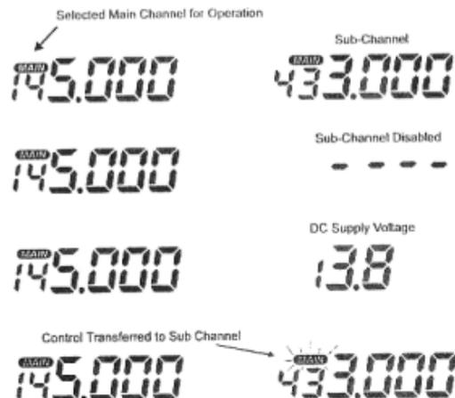
There are three ways to select or toggle a band for operation. You can *momentarily* press in the VOL knob to select the band you want as the main channel, or else momentarily press the DIAL knob or **PWR** button to toggle the main band of operation. Remember to only press these for less than 1/2 sec, as holding them longer will turn the transceiver off, or activate other functions.
