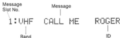
abled and **MSG FULL** appears after the ninth message (see page 67). To view messages, press **MSG** and recall message slots using joystick (up/down), the DIAL knob or **A/B** keys. Empty message slots are indicated by **<BLANK>**.
