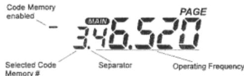
In addition, one touch of the **A** and **B** keys now select *code memories*, instead of tuning or scanning as before (D/MR operation remains unchanged). Each press displays the selected code memory setting for a second, then returns to the channel display.
